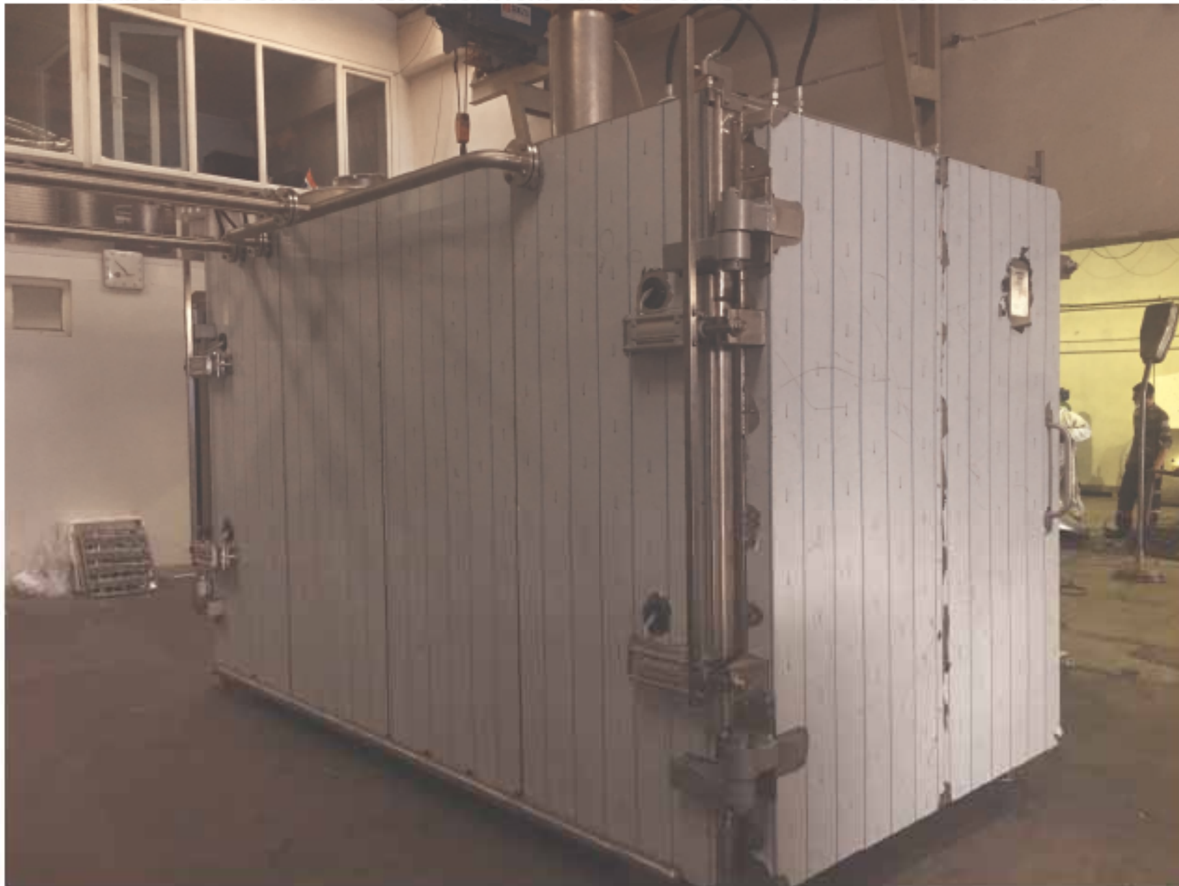
15 M3 DOUBLE DOOR VIEW – PNEUMATIC PISTONS – CHANNEL CONNECTIONS – INSULATION – BUFFERING TANK
