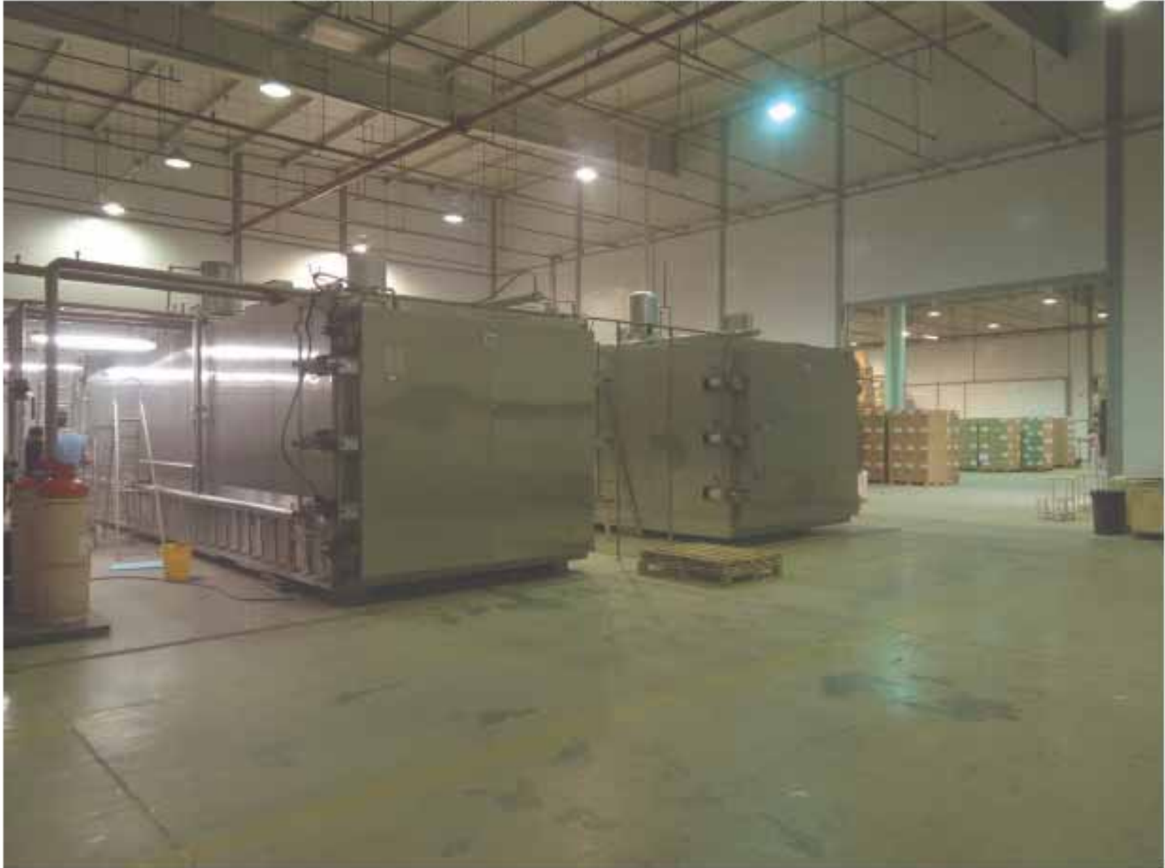
TWO UNITS OF 62 M3 STERILIZER VIEW DOUBLE DOOR
