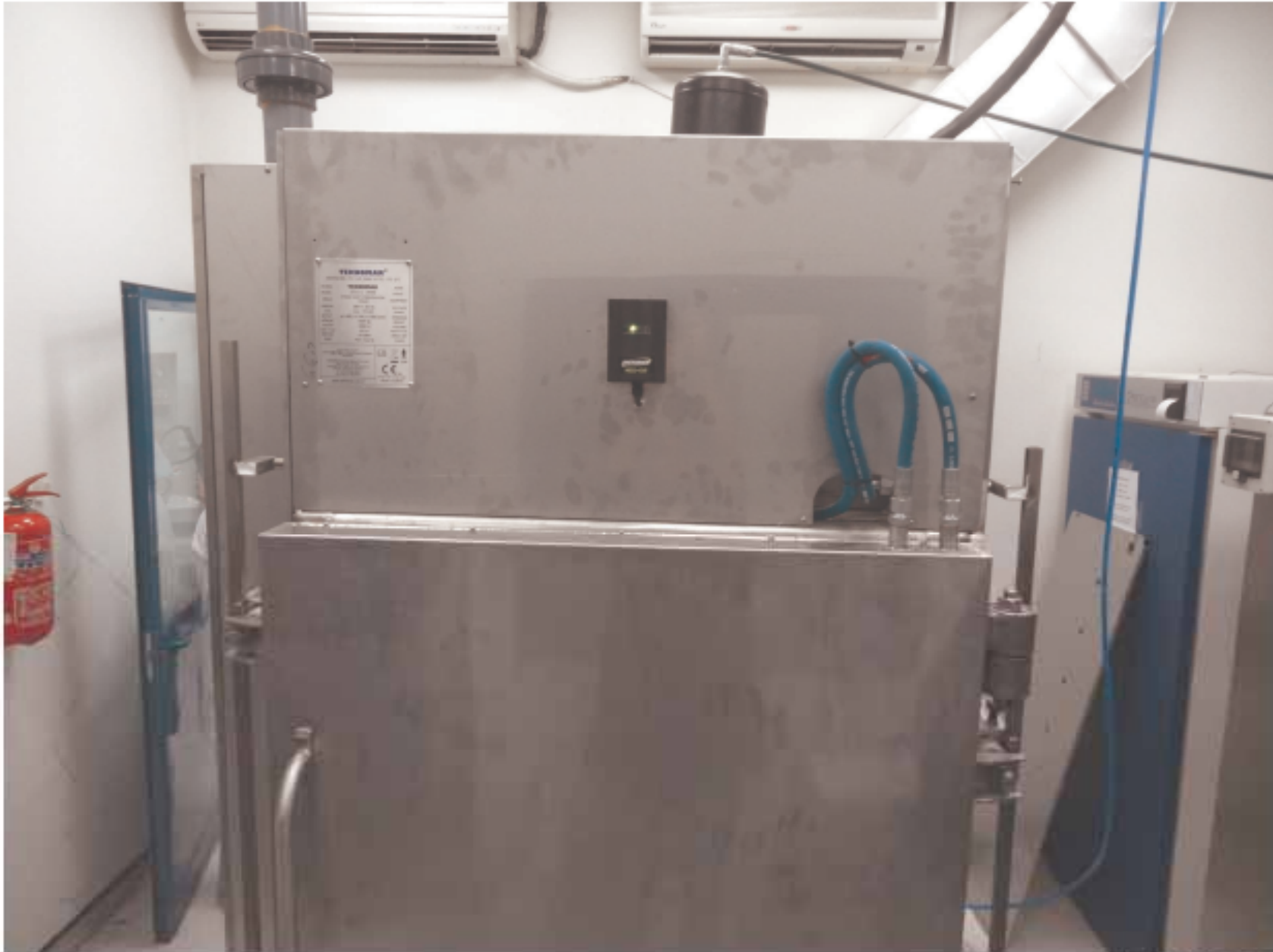
SUTURE STERILIZATION – DOUBLE DOOR – EXHAUST CONNECTION – EO DETECTOR SAMPLE VIEW
