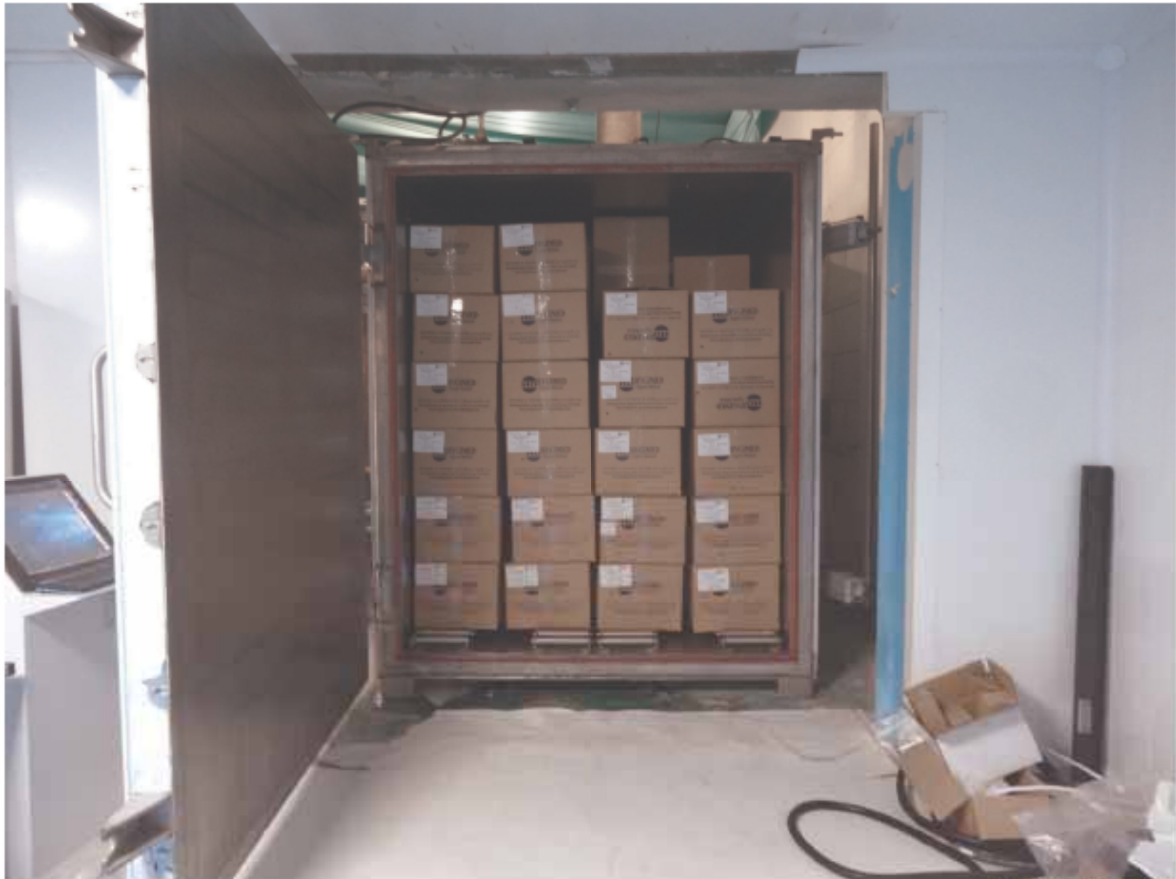
15 M3 STERILIZER – FULL LOAD – SINGLE DOOR
